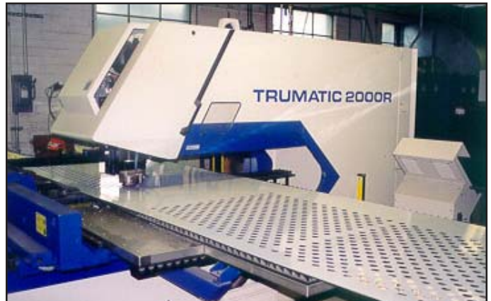
The TRUMPF 2000 punches the perforated louver “skin.”
